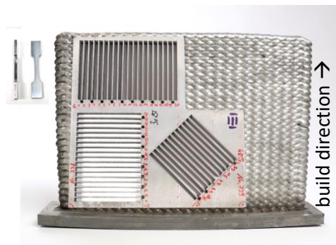
Figure 1: Specimen orientation and locations of the single path WAAM wall
